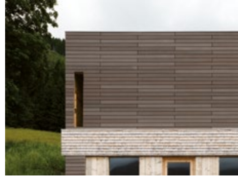
öko skin flex 125 mm, terra, horizontal installation (1/2 shifted), screwed on wooden substructure
